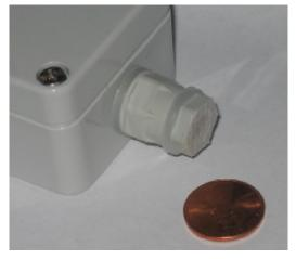
In the photo above, the SHT75PG is mounted on a sealed polycarbonate enclosure. The sensor element itself is protected by the gore-tex membrane making it permeable only to water vapor. The enclosure could hold a data logger or transition wiring to a cable.
