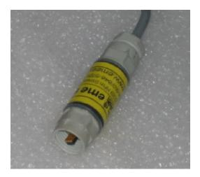
The SHT75PG/3M above is mounted on a length of 3/8" PVC pipe. Connection is made to a three meter cable that terminates in four tinned wires. This unit is shown with the protective cap removed for fastest response. Observe that the open PG7 guards the sensor from breakage, but allows for good air flow.
