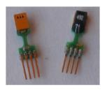
The basic SHT75 comes in a SIP package that features a long neck for low thermal mass, a flow-through air path for fast response, and pins on 0.05" centers.
