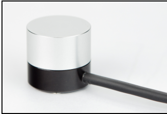
Figure 6-3. Sensor Base Cover installed on the sensor base in place of the sensor head.
