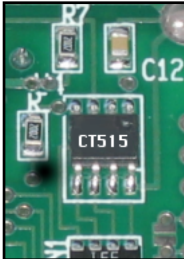
Figure 2: The photo shows the CT515 in the 8 pin soic package mounted on a circuit board. The components around it on the board are the bypass capacitor, the pullup resistor for the data line, and the protection resistors in an array package. The inputs lead to Phoenix terminals on the other side of the circuit board.
